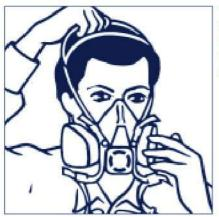
1. Place the respirator over the mouth and nose, then pull the harness over the crown of the head.
