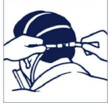
4. Tighten bottom straps using either front or rear adjustments. (Strap tension may be decreased by pushing out on back side of buckles).
